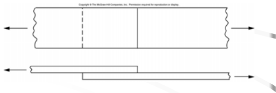
Fig. 1-9 A simple lap joint
