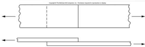
Fig. 4-6 Design of a simple lap joint
