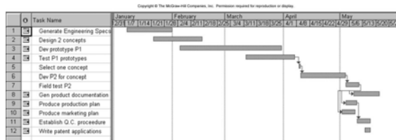
Fig. 5-4 Gantt chart for BikeE suspension system project
